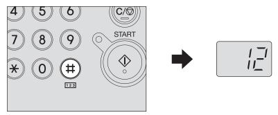
2 Switch the display to check the rest of the total number.
